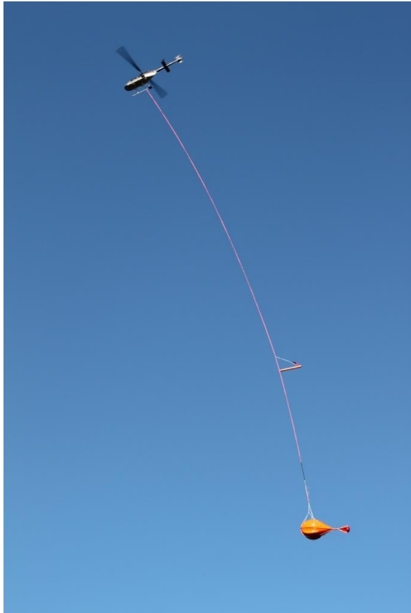
Image 1. Expert Geophysics Limited's MobileMT system on survey
